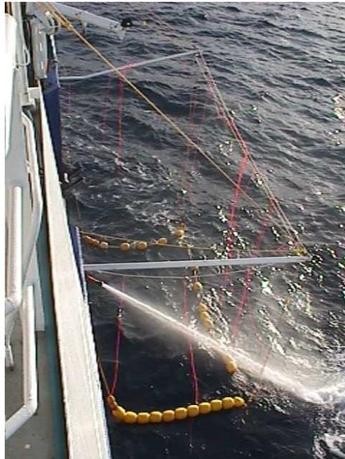
Figure 3: Bird Excluder Device used on the FV *Janas*.
