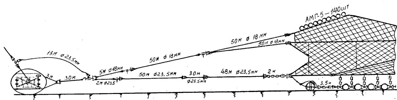
Figure 3: Rigging of trawl "Khek-4M".
