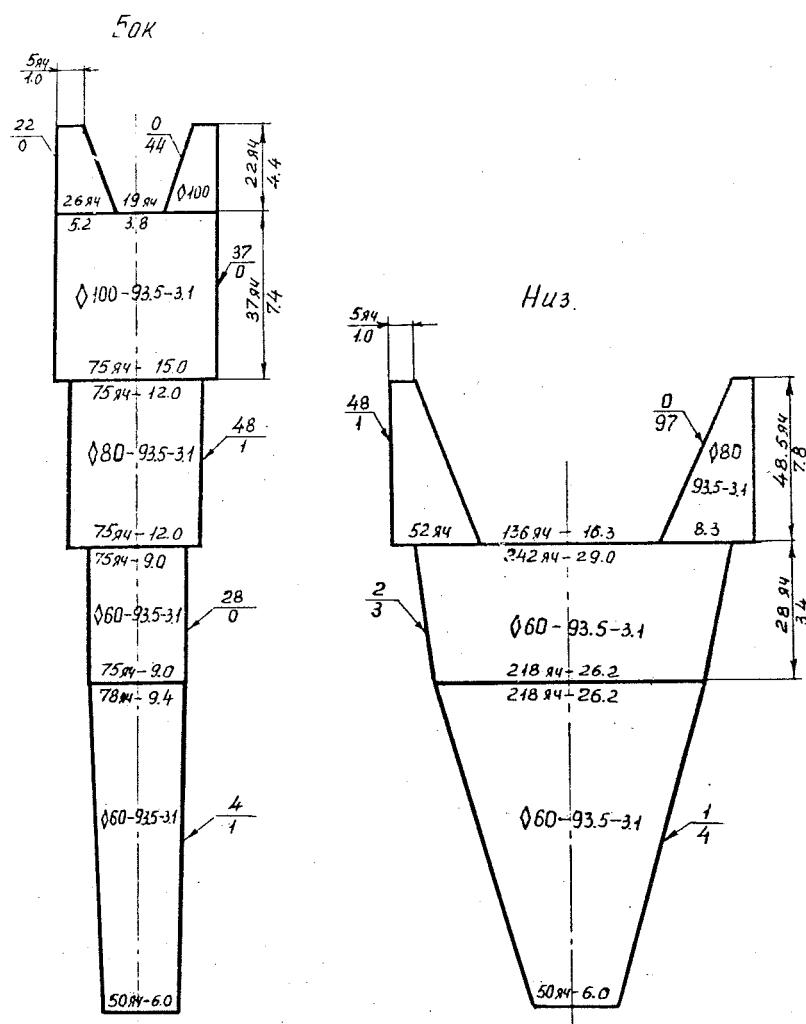
Figure 2: Side and bottom panels of trawl "Khek-4M".
