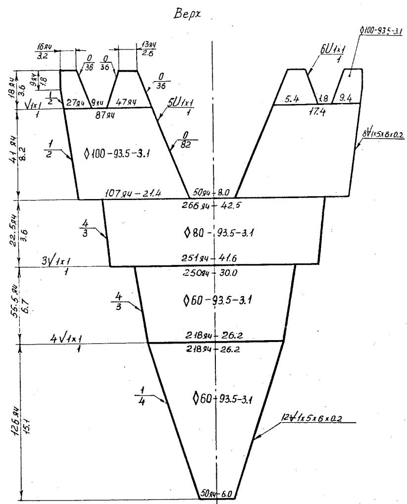
Figure 1: Top panel of trawl "Khek-4M".
