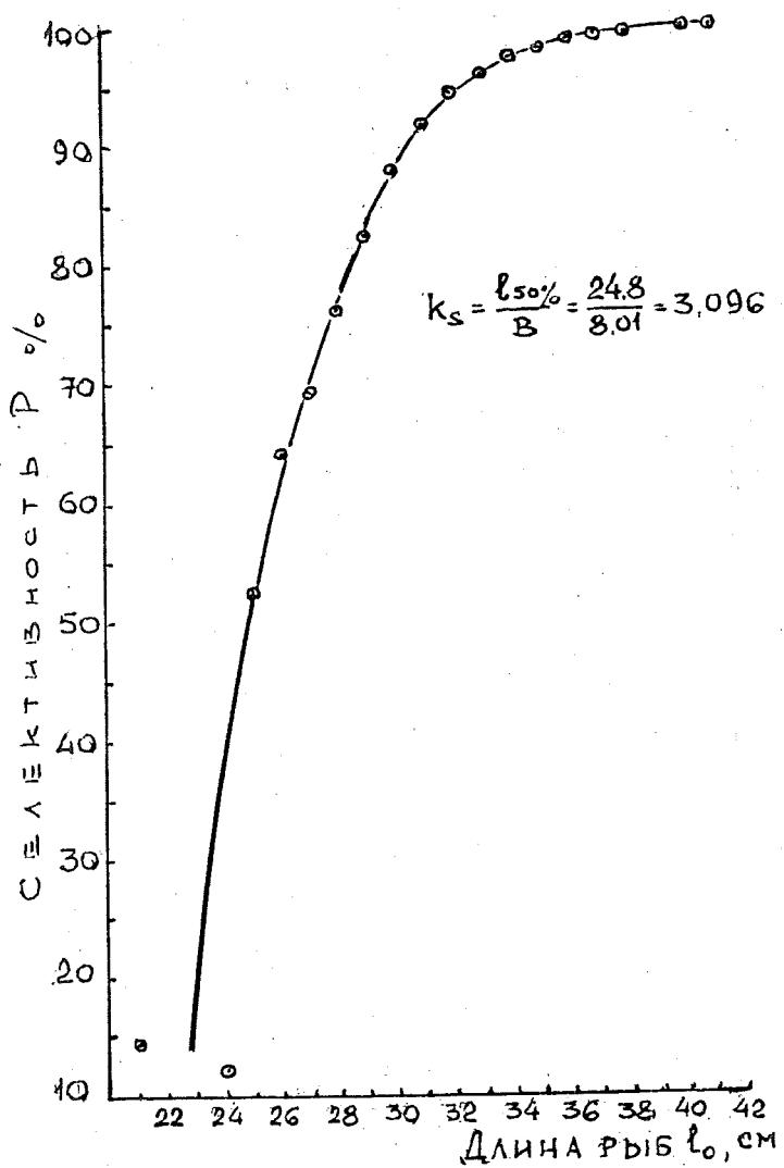
Figure 4: Selectivity curve for trawl bag with mesh size  $B=80.1$  mm in respect of *C. gunnari* on the South Georgia Shelf (BMRT *Anchar*, June 1990. Number of hauls  $N=29$ . Calculations made using the method of sliding mean).
