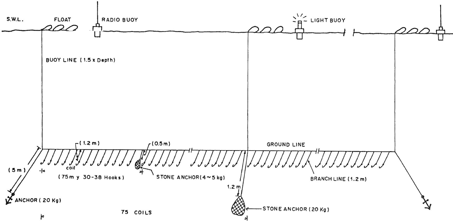
Figure 1: Configuration of bottom line used by *Friosur V* for capture of *D. eleginoides*.
