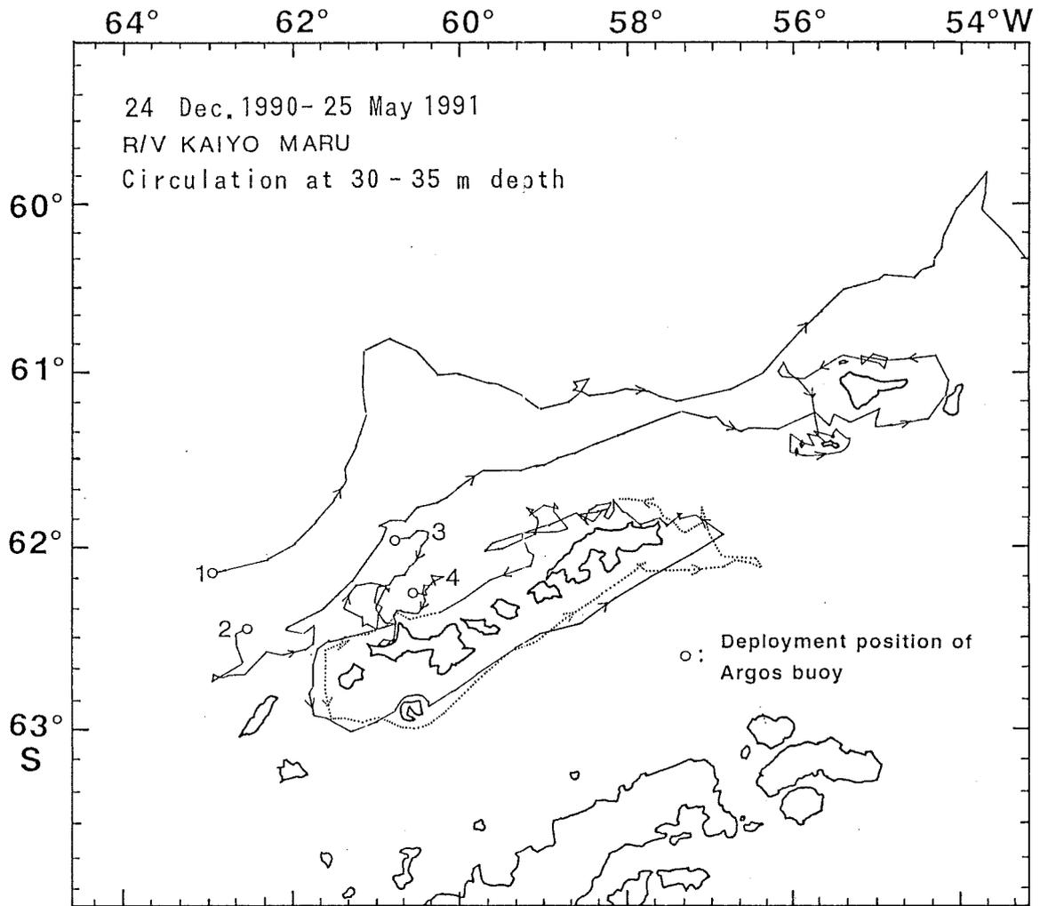
Figure 7: Water circulation at 30 to 35 m depth derived from the paths of four satellite-tracked buoys. Since Buoy 3 drifted more than one and a half circulations around the South Shetland Islands, its second circulation is shown by dotted line.
