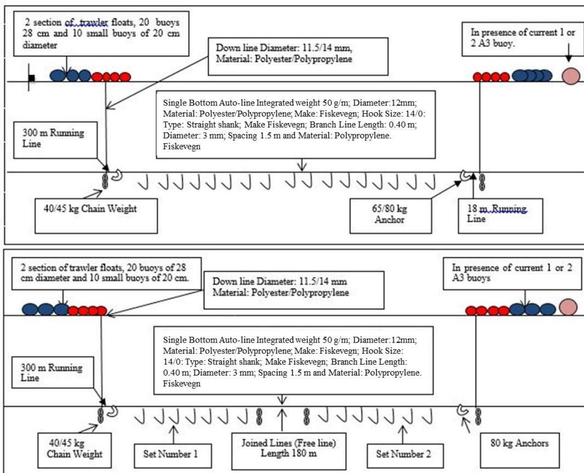
The vessel uses two different gear configurations depending on the topography of the fishing grounds and the ice conditions, single lines and join lines, as illustrated above.
