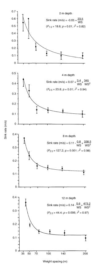
Figure 3: Longline sink rate to depths, shown as a function of weight spacing (WS in metres) on longline set by the *CFL Pioneer*. Results to 2 m depth are provisional (see text). Note differences in increments on 'y' axes. Closed circles indicate means ±1 standard deviation for three dive recorders deployed simultaneously on longlines.
