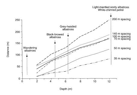
Figure 8: Distance astern at depths, shown as a function of weight spacing on longline. Maximum recorded diving depths of grey-headed albatrosses, light-mantled albatrosses and white-chinned petrels are indicated by dotted lines. For given weight spacings, cross reference of seabird diving depths and 'y' axis reveals distance behind the *CFL Pioneer* baited hooks are 'available' to birds.
