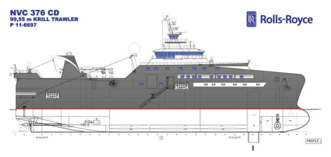
Figure 1: The new krill vessel with an instrument drop keel (1) and a hangar for operation of ROV and oceanographic and biological sampling gears (2). The vessel is 99 m long and has diesel electric propulsion.
