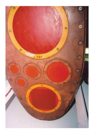
Figure 2: The tip of the drop keel with six acoustic frequencies (from RV *G.O. Sars*). The intention is that the tip can be demounted and replaced by another module with tailored sensors in accordance with cruise objectives.
