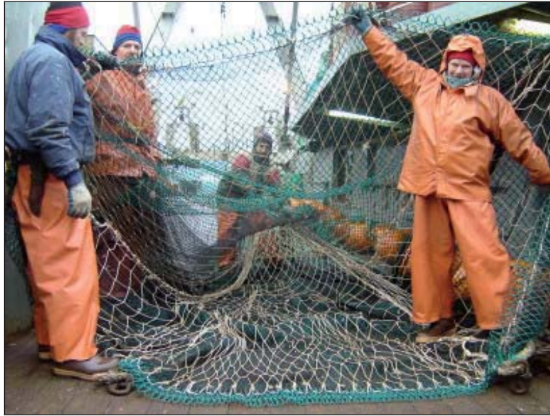
Figure 5: Mesh funnel spliced into the inner panel on the Top Ocean .
