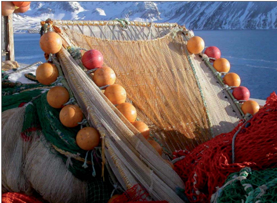
Figure 1: Seal-exclusion device on the Atlantic Navigator .
