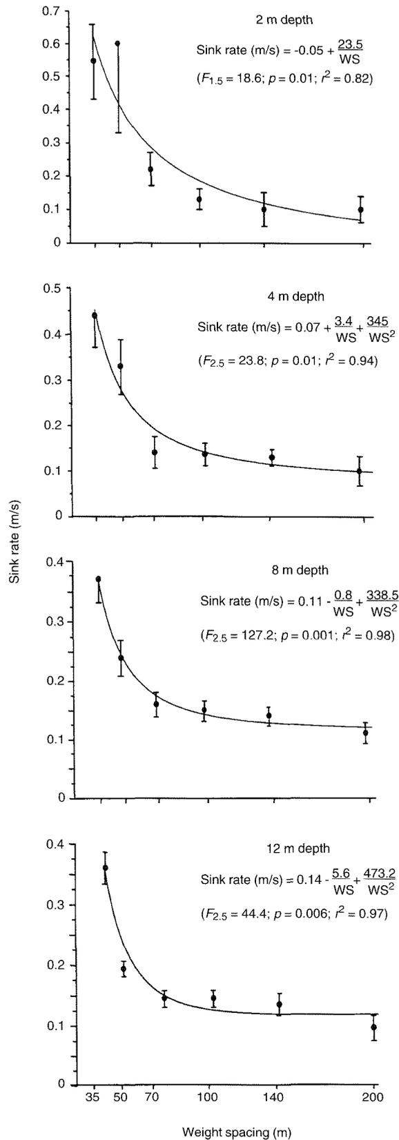
Figure 3: Longline sink rate to depths, shown as a function of weight spacing (WS in metres) on longline set by the CFL Pioneer. Results to 2 m depth are provisional (see text). Note differences in increments on 'y' axes. Closed circles indicate means  $\pm 1$  standard deviation for three dive recorders deployed simultaneously on longlines.
