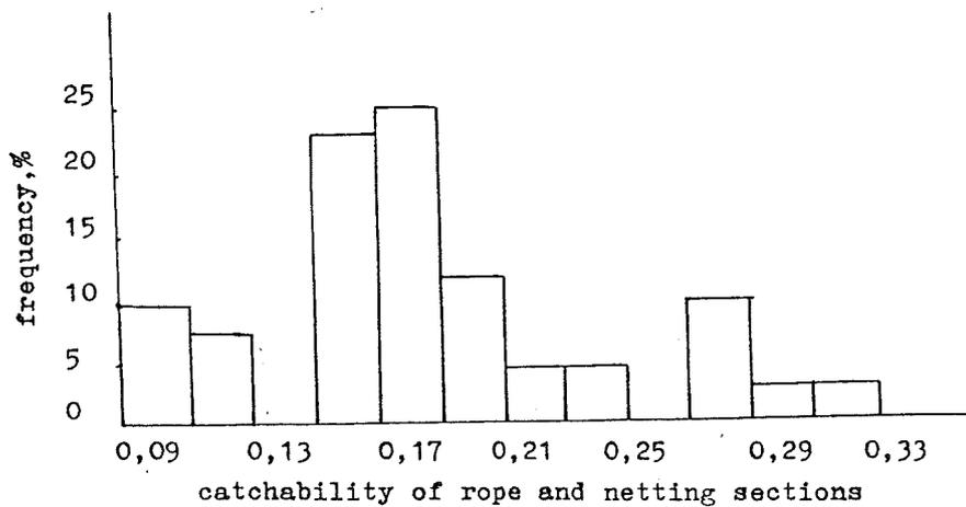
Figure 3: Histograms of distribution in relation to the catchability rate of the 72/308 trawl from targeted krill concentrations in the Elephant Island area in January 1985. (Hydroacoustic data).
