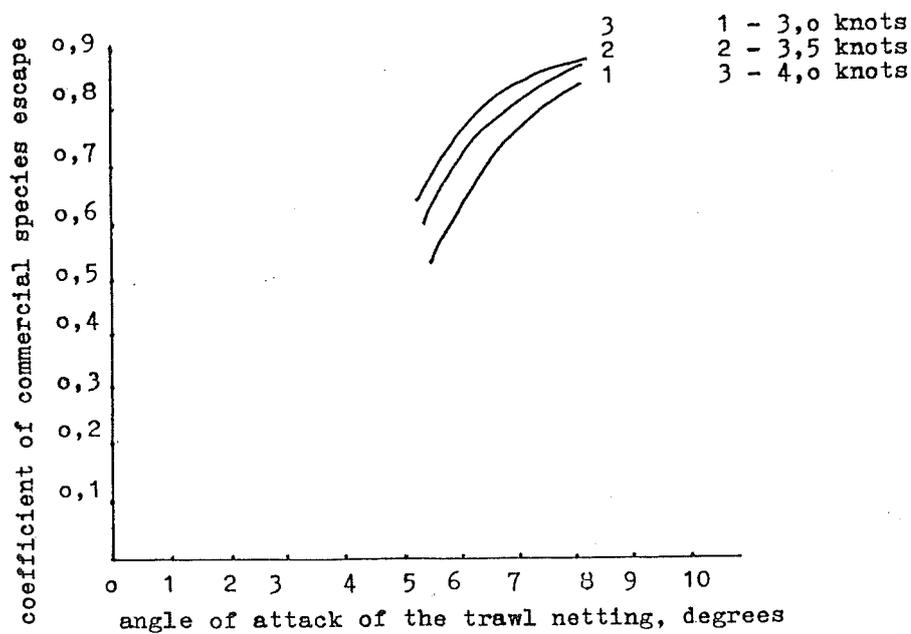
Figure 2: Relationship between total catchability of the 72/308 trawl, trawling speed and netting angle of attack according to hydroacoustic data.
