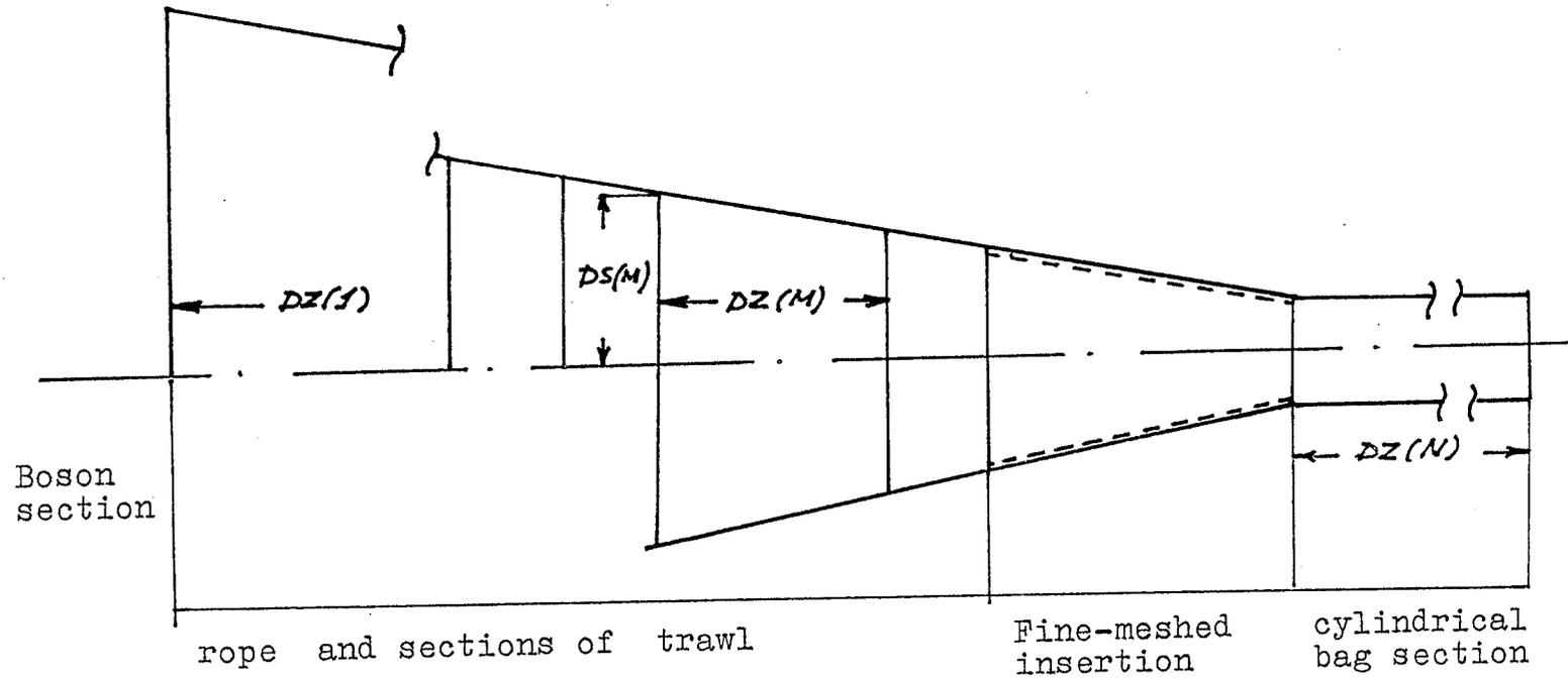
Figure 7: Design of trawl sections.
