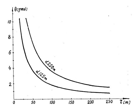
Figure 3 Dependence of the depth of detection of individual krill for different ranges of the recorder on transducer threshold directivity angle.
