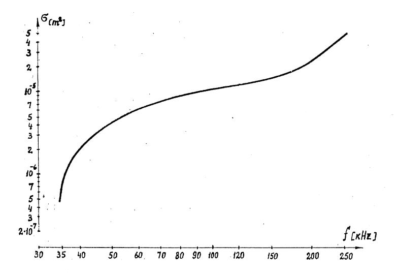
Figure 1 Dependence of freshwater shrimp acoustic section on frequency (shrimp length - 4.5 cm).
