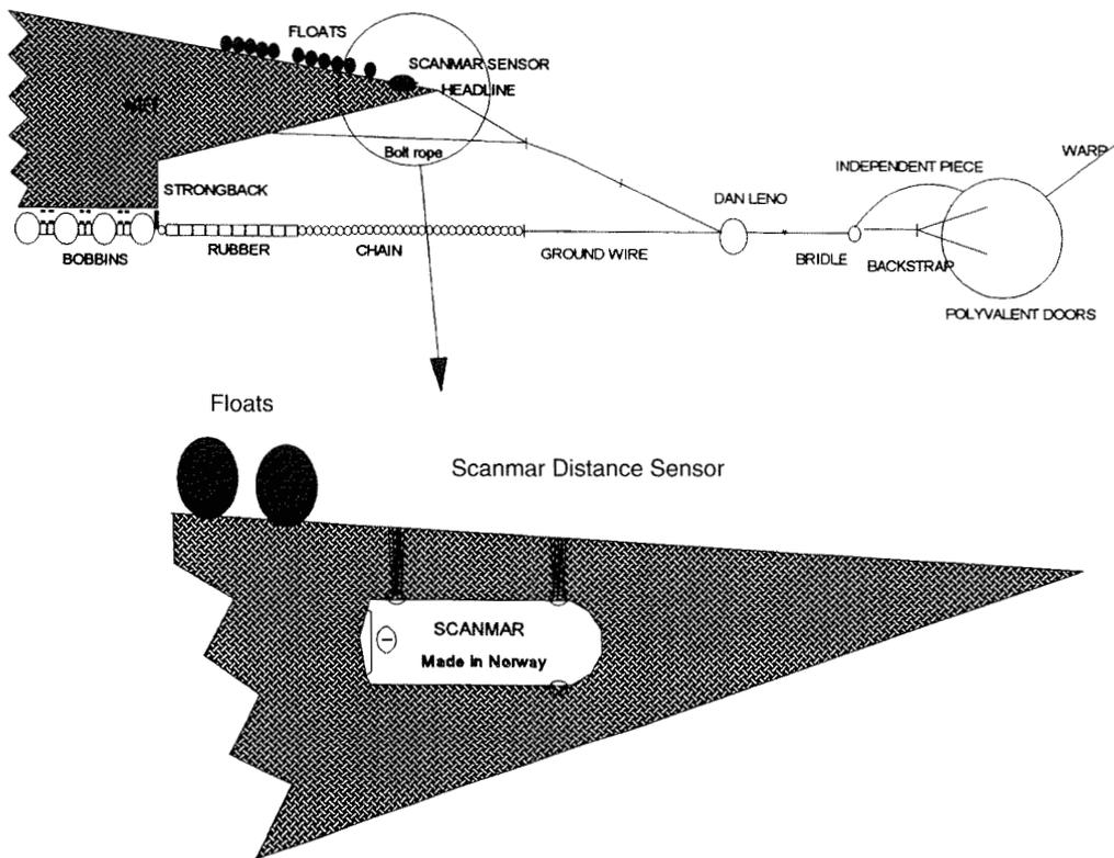
Figure 2b: The positioning of the Scanmar sensor on the FP-120.
