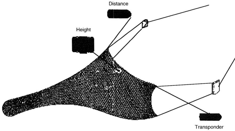
Figure 2a: The positioning of Scanmar sensors on a bottom trawl.
