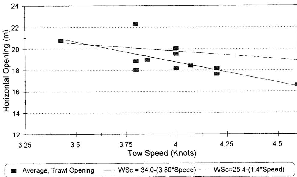
Figure 13: Regressions of horizontal opening against tow speed (old and revised equations).
