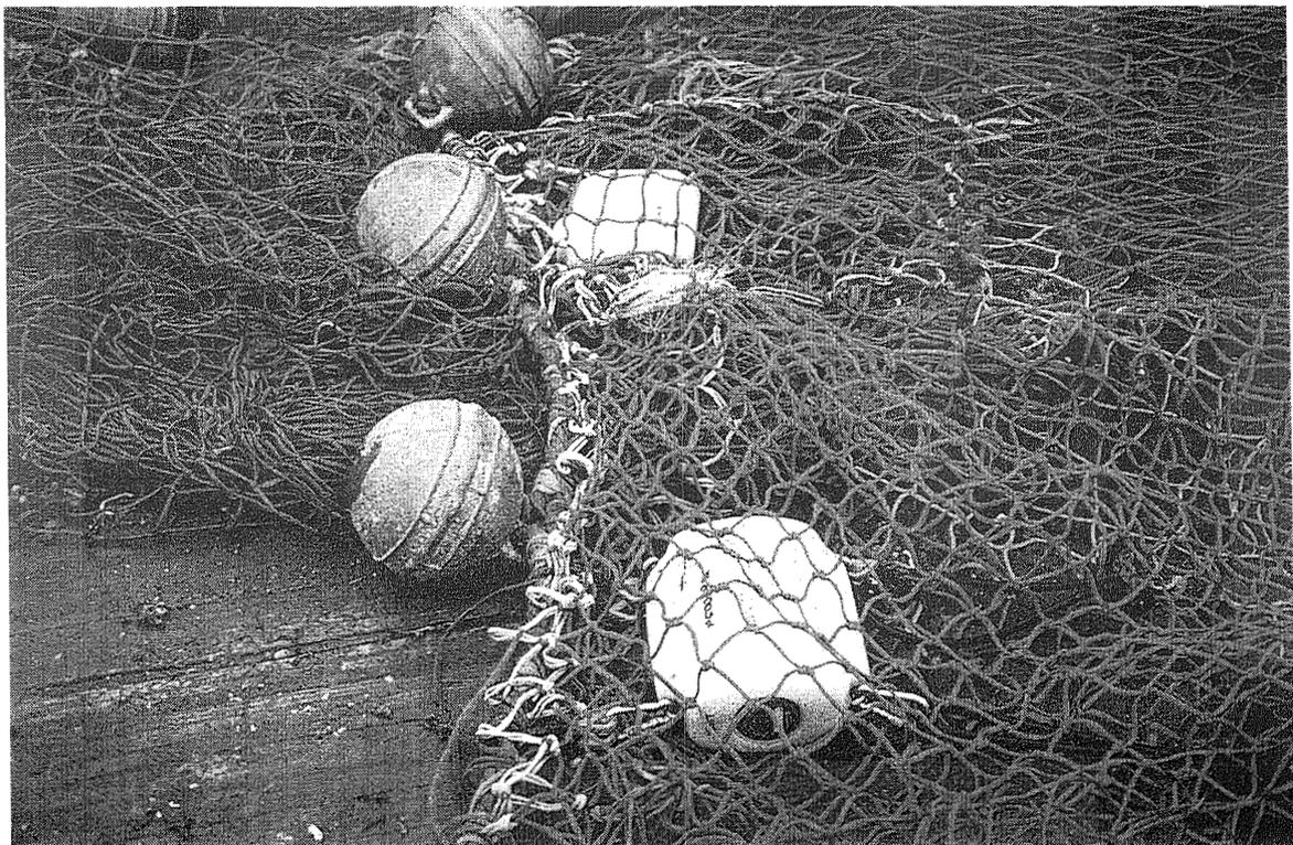
Figure 4: Photograph of the fixing of the Scanmar sensors on the FP-120.
