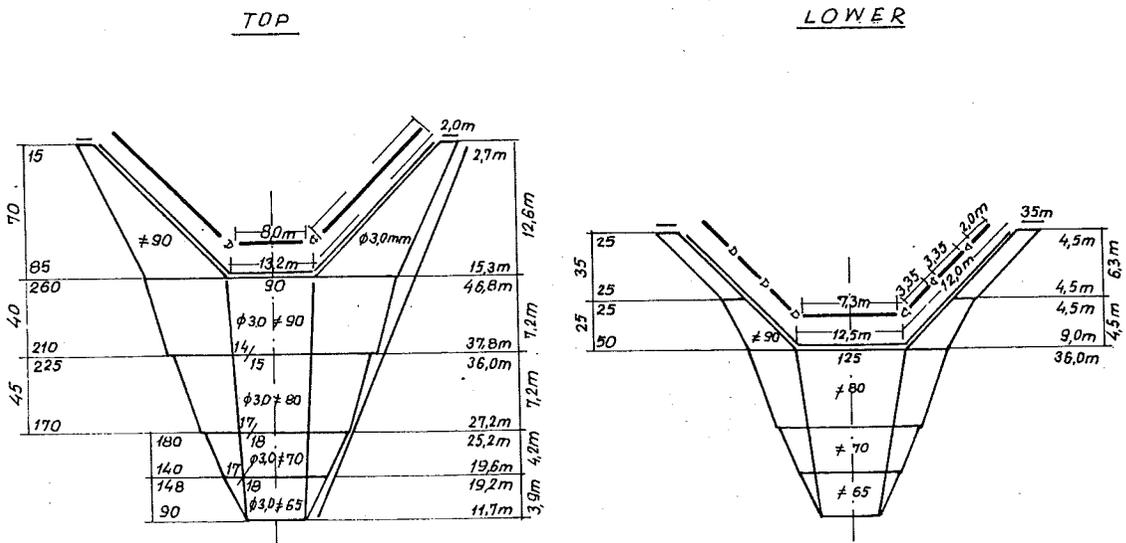
Figure 2 Plan of 32/36 bottom trawl construction.
