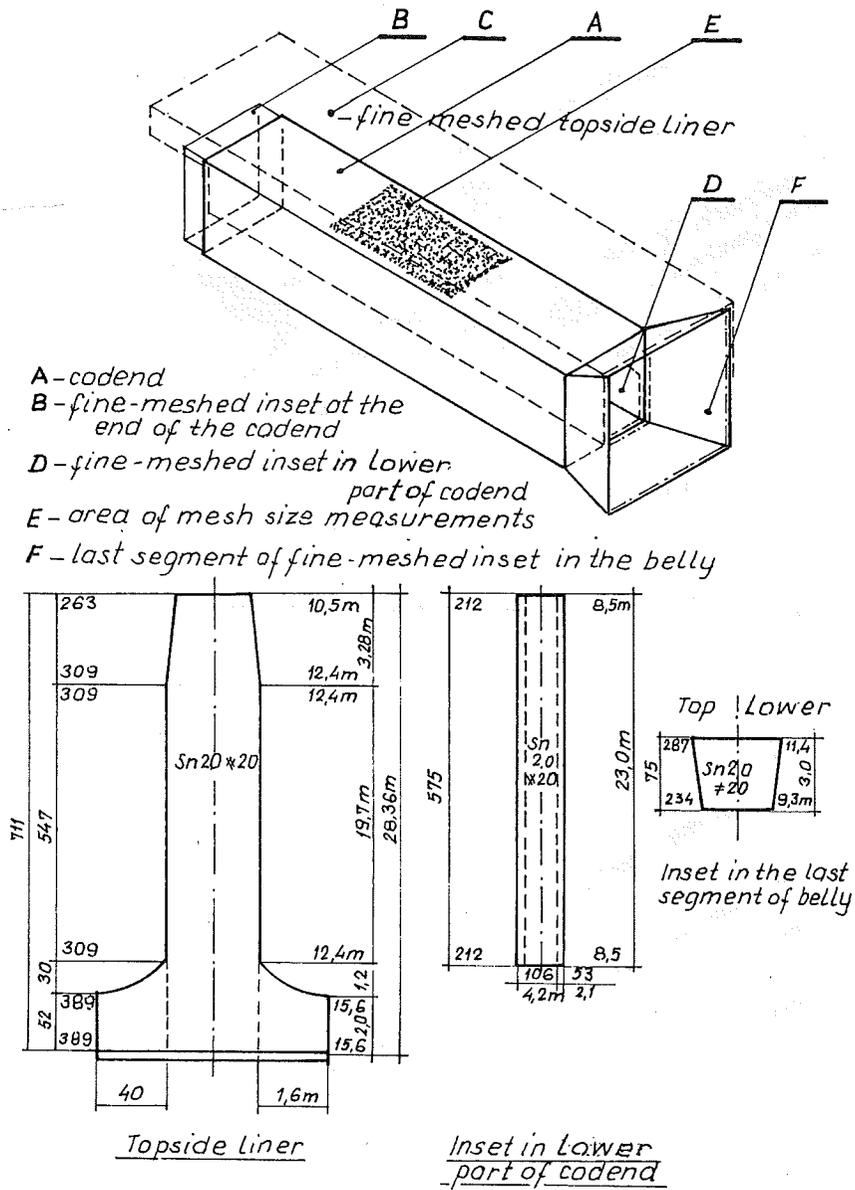
Figure 4 Plan of tape codend with fine-meshed topside liner and fine-meshed inset in lower part of codend.
