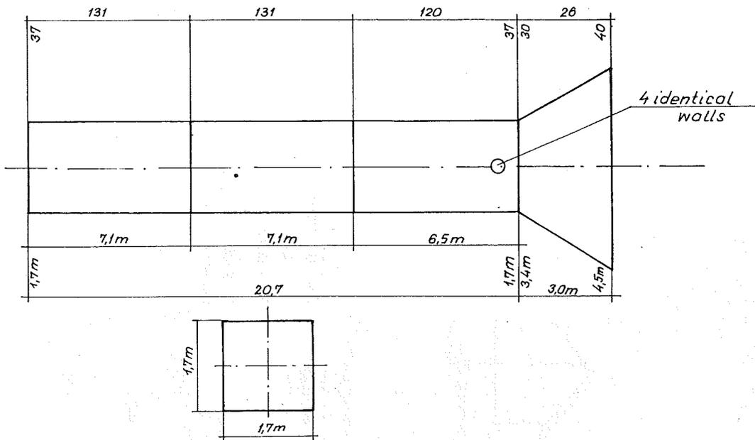
Figure 1 Plan of tape codend construction.
