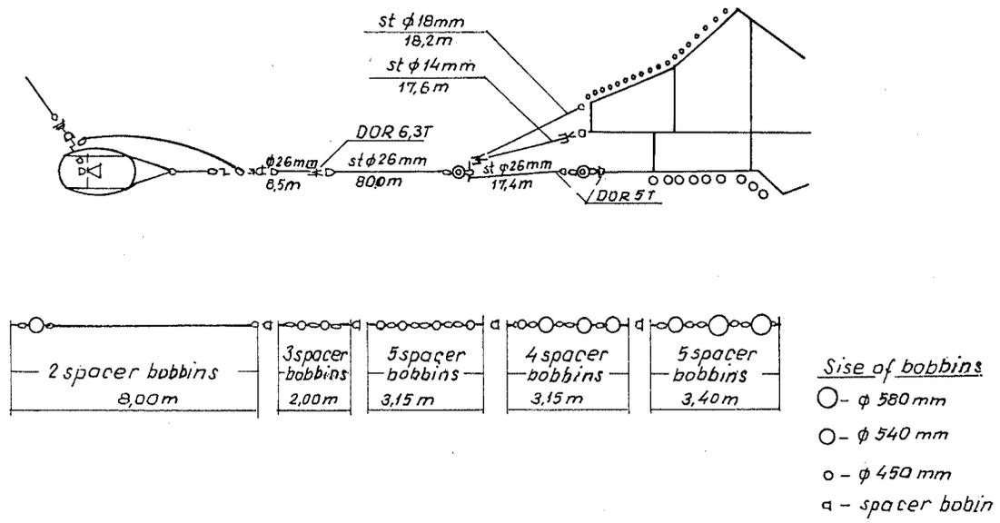
Figure 3 Plan of gear rigging for 32/36 bottom trawl.
