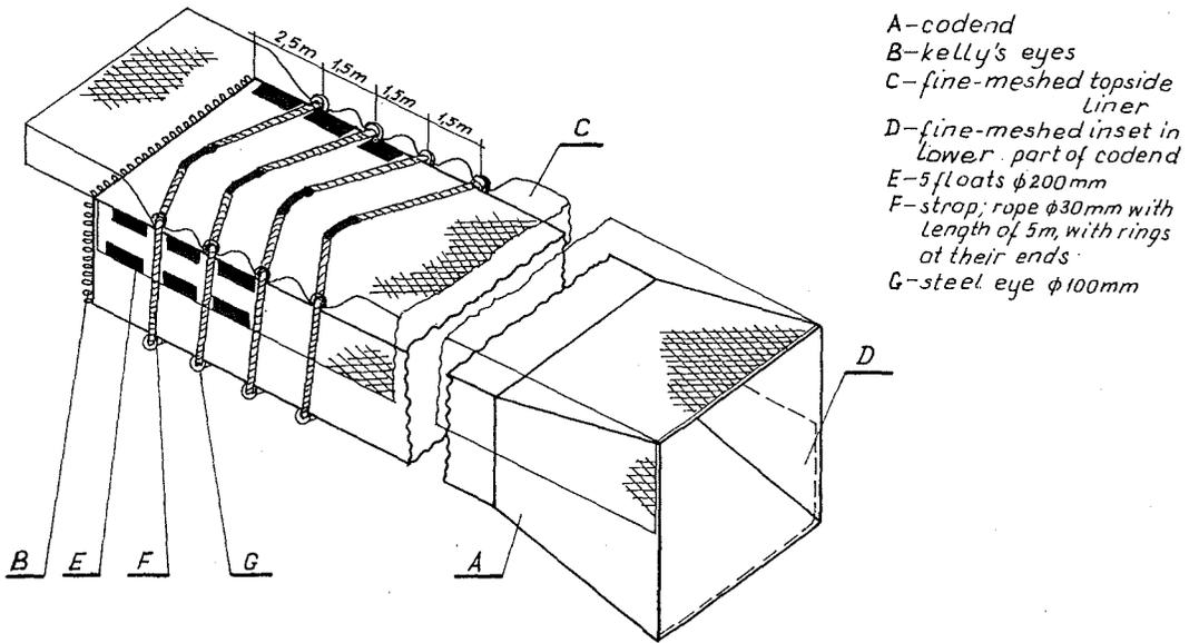
Figure 5 Plan of standard codend rigging (version I).
