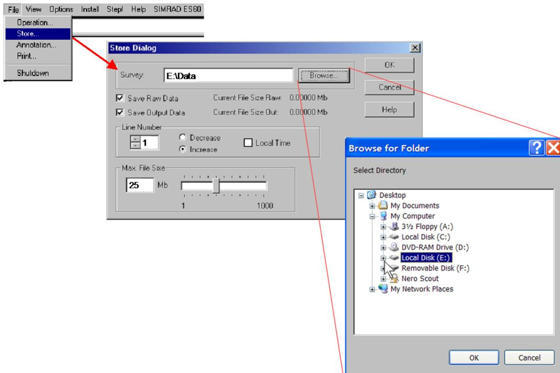
**Tip:** USB drive letter will not be C and is unlikely to be D, and is probably E on most installations. Supplied drives will most likely have a folder \Data. If so, log to this folder, i.e. E:\Data\*.
